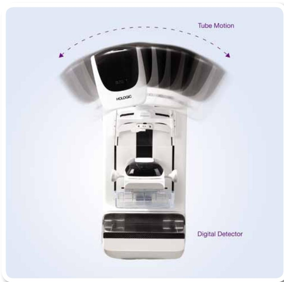
When a screening exam is performed in combo-mode, the breast is compressed in the normal way. The x-ray tube first sweeps in a 15-degree arc over the breast, acquiring a series of 15 low-dose projection images at multiple angles. These projection images form three-dimensional reconstruction.
