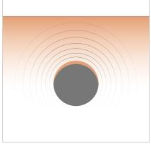
The rapid, local laser effect causes a big expansion, which creates acoustic shock waves.
